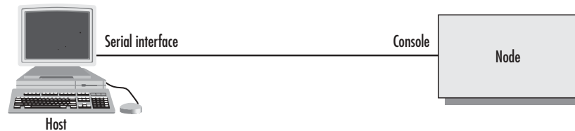
Figure 6. Setup for initial configuration via the console port
