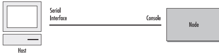
Figure 9. Setup for initial configuration via the console port
