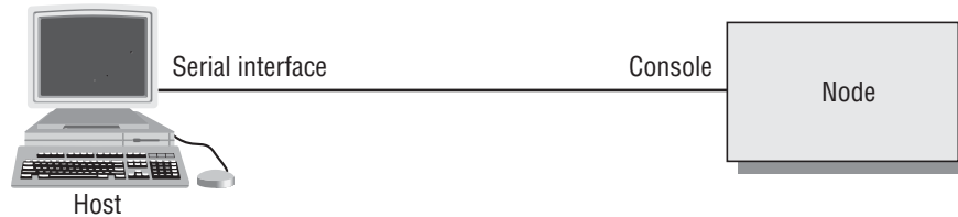
Figure 6. Setup for initial configuration via the console port
