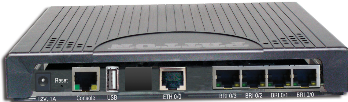
Figure 2. SN4130 Rear Panel
