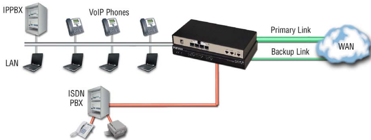
Figure 7. WAN uplink redundancy
