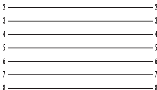
Figure 14. Typical Ethernet straight-through cable diagram for 1000Base-T
